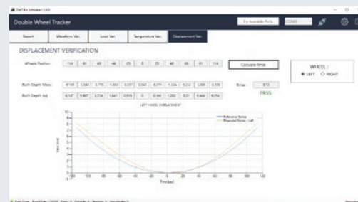
Rut depth verification with shaped specimen
