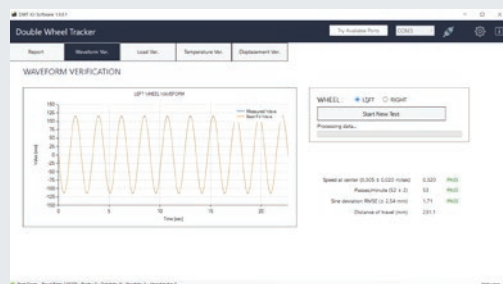
Sinusoidal movement verification
