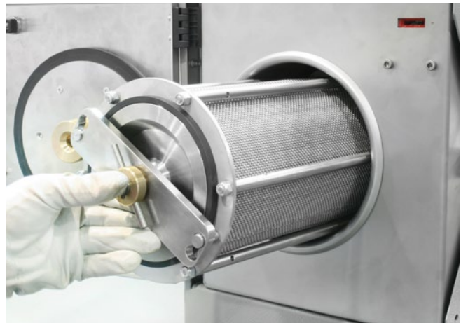
Placing the washing drum into the machine
