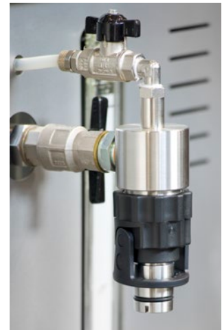
Detail of 75-PV5 X100 fast connection for Rotary evaporator flask, for bitumen solution sampling
