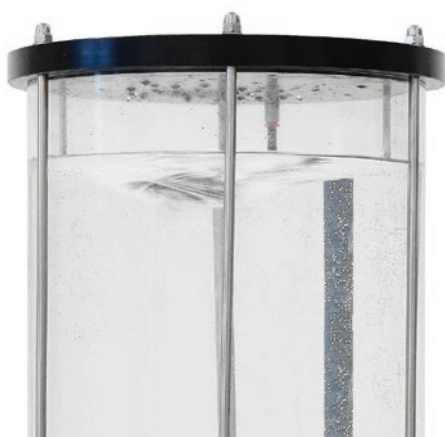
Initial water vortex during cavitation and vacuum application
