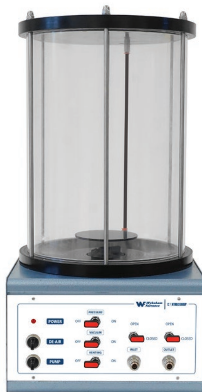
Standalone all-in-one de-airing system
