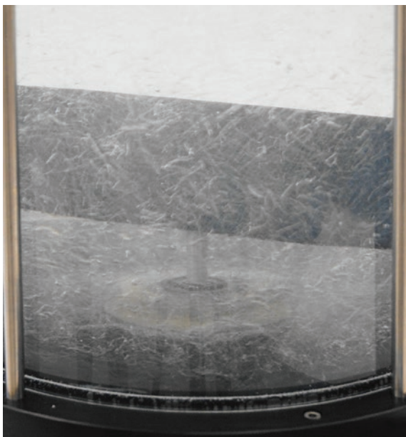
Detail of cavitation system, it allows water to be de-aired much faster than when only using vacuum
