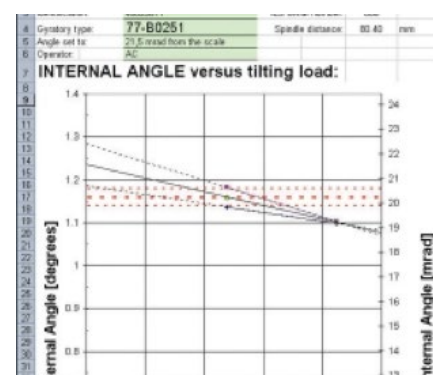
Calibration certificate obtained with the 78-PV0255 ILS apparatus, using the Macro
