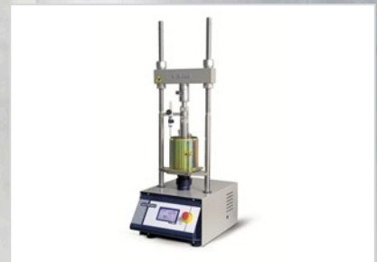
Bearing capacity: CBR, Proctor, Marshall and plate bearing
