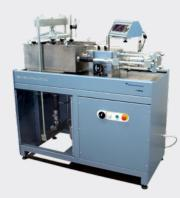
stepper motor. A microprocessor unit manages the test steps whilst automatically recording force, axial pressure and displacements.
