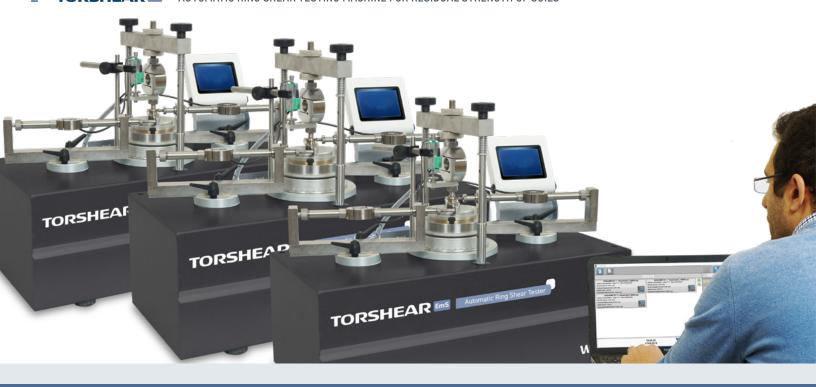
Torshear EmS is a versatile and fully automatic ring shear testing machine that benefits from the new low maintenance, efficient and environmentallyfriendly Electromechanical Servoactuation (EmS) technology.
