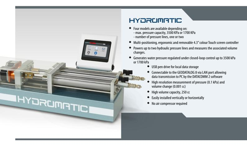
Hydromatic standalone is a general-purpose water pressure source and volume change controller. It is driven by a stepper motor, which enables the unit to measure the volume change. The unit consists of a hydraulic piston, driven by a ball-screw and gearbox, mounted on a low friction-slide, and is managed under closed-loop control by the built in data acquisition and 4.3" touch-screen colour control panel.
