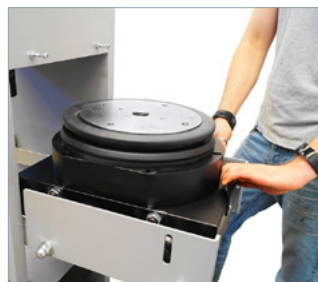
Detail of the upper block platen and spherical seat sliding off by solid rail system
